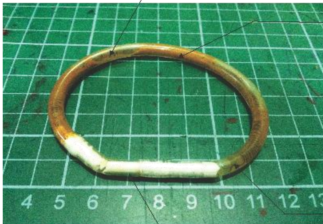
Syringe Plastic Cylinder with Teflon to seal the Gans Mix
